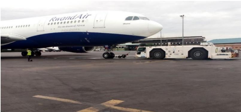
*Fig 5. Pushing back an Aircraft*
